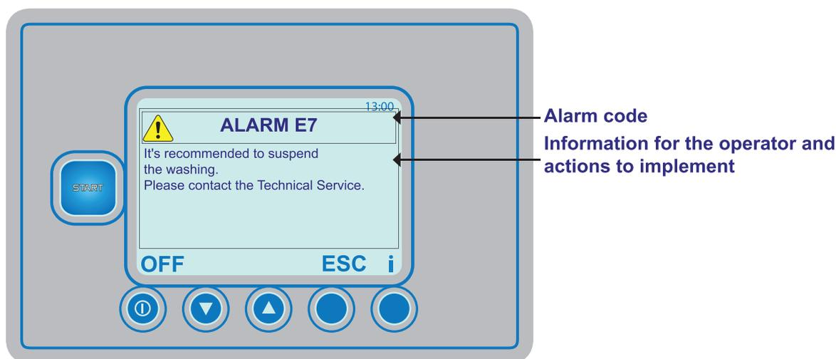
If the alarm does not block the machine it is possible to continue the operation by pressing **6 ESC** key. The machine will continue to signal the alarm until the resolution of the problem by:
